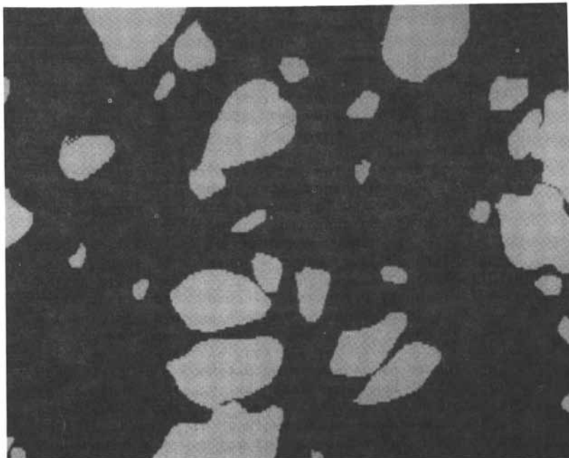
Figure 3: A binary image obtained by edge detection and segmentation of Figure 2.
